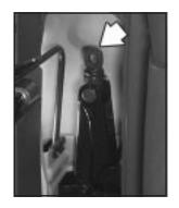
2. Turn the jack screw to remove the jack from the clamps. If the screw is too tight, use the jack handle to loosen it.
